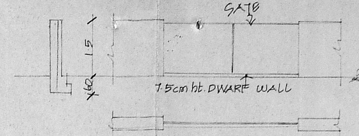
COMPOUND WITH DWARF WALL DETAIL
